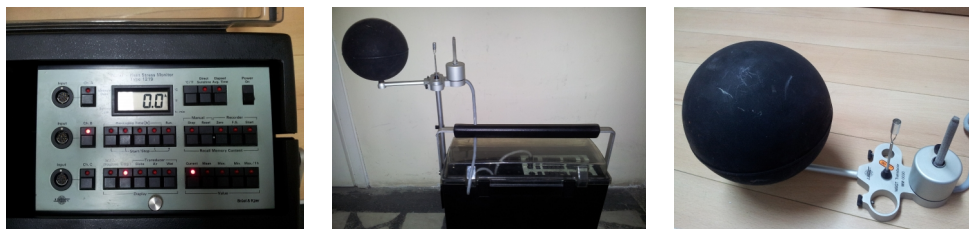
Slika 1. Heat stress monitor Brüel-Kjær type 1219, sa odgovarajućim davačem MM 0030 Picture 1. Heat stress monitor Brüel-Kjær type 1219, with transducer set MM 0030
