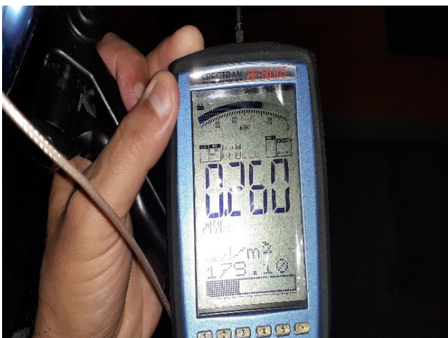
Picture 3a. Example of measuring the electric field strength using the instrument Spectran HF 60105
