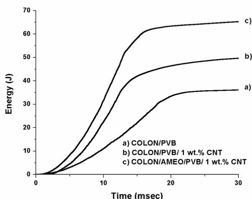
Figure 20 - Energy versus time for all the samples
