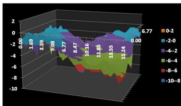
Figure 13 - Indentation depth analysis of the shot No. 1
