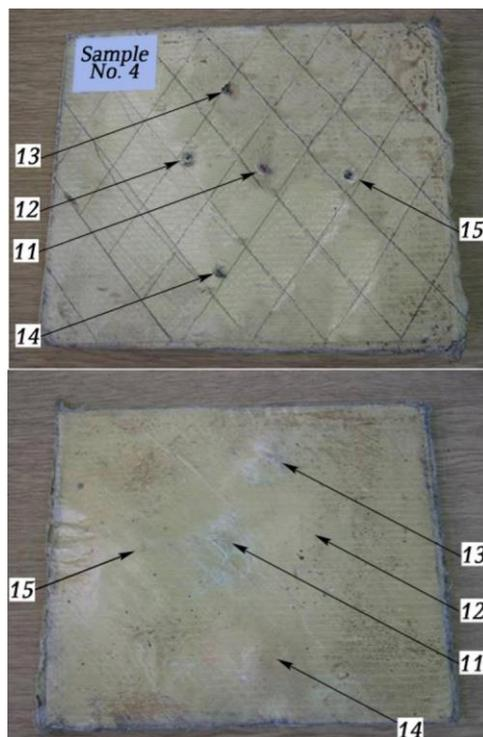
Figure 11 - Front and back side of shot sample No. 4
