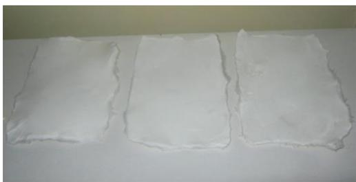
Figure 2 - The coated aramid fabrics with deposited PVB-SiO<sub>2</sub> fibers
