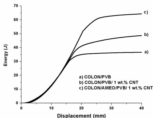
Figure 21 - Energy versus displacement for different Colon/PVB fabrics
