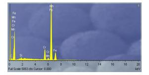
Figure 5. EDS spectrum at point 1
