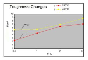
Figure 2 Diagram of toughness changes Slika 2. Dijagram promene rastegljivosti
