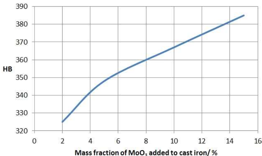
Figure 5. Measured Brinell hardness of the iron alloy samples as a function of \text{MoO}_3 mass fraction
