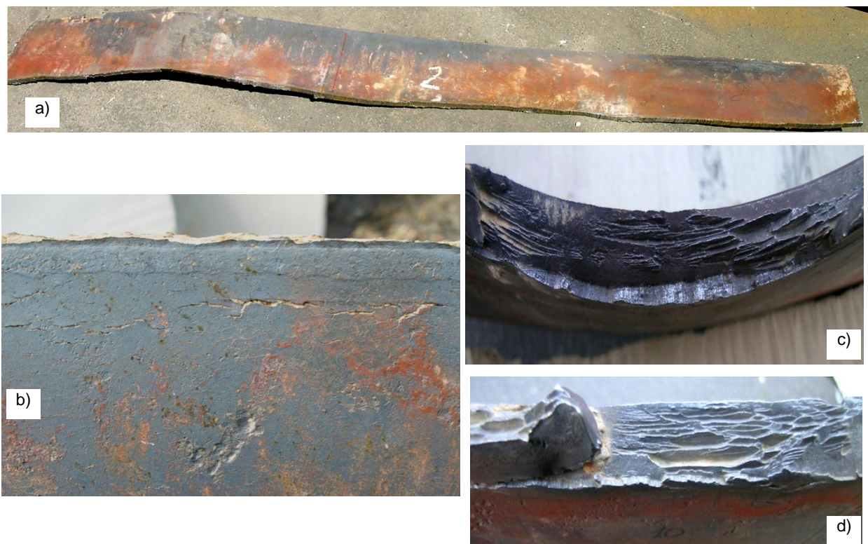
Figure 4. The fragment of broken pipe A (templet 2): a – appearance; b – cracks near the broken edge; c, d – stratification in the rupture
