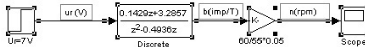
Fig. 8. Simulink model of the system with parameters calculated by identification of the system.
