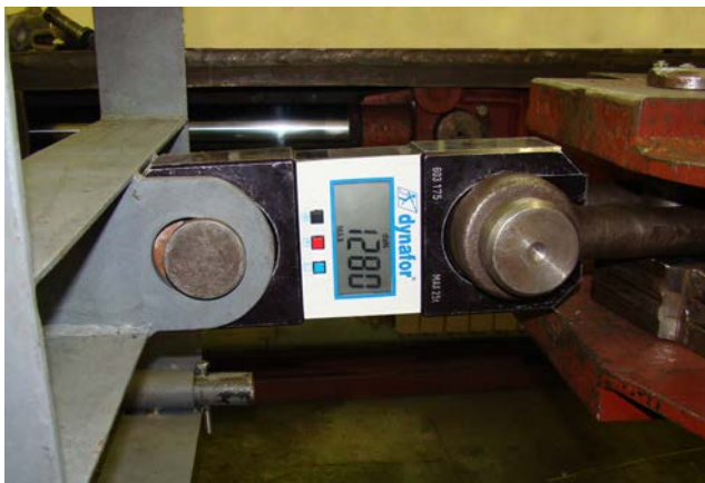
Figure 5. Display of measurement during stiffness test - value of force in decanewtons that corresponds to a 3 % deflection of one of the pipe sample inside diameter
