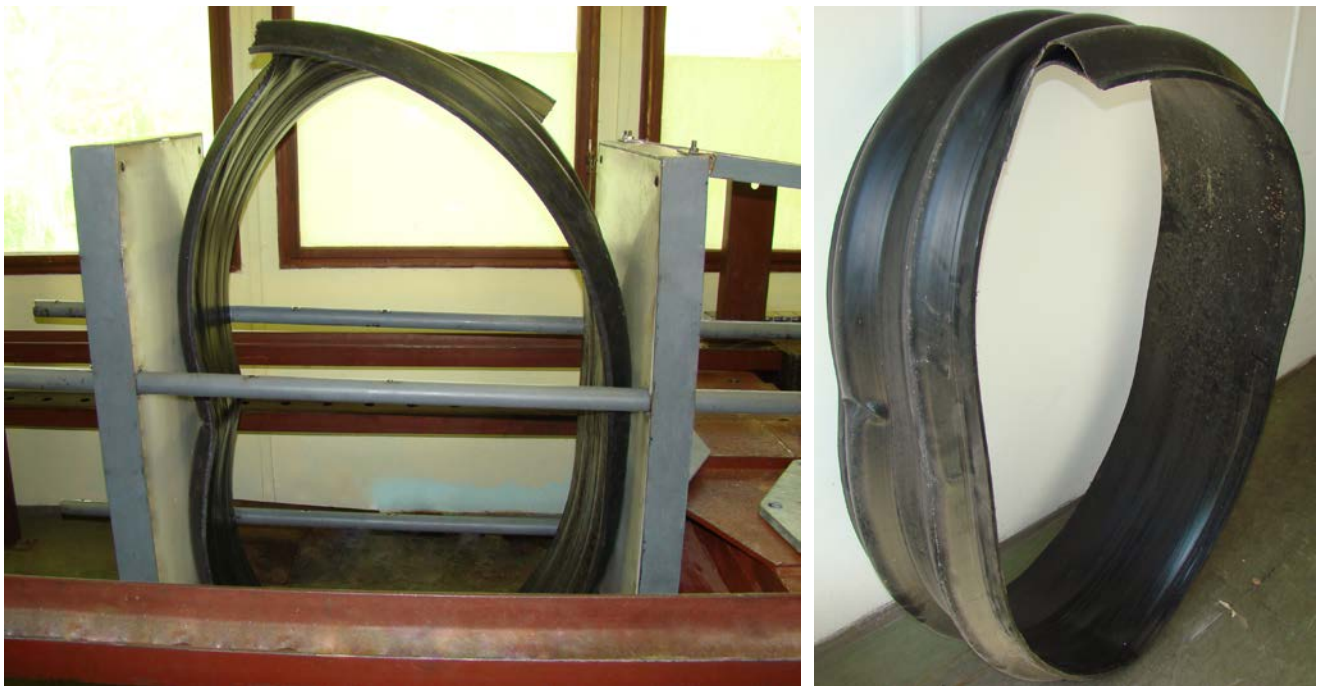
Figure 7. The flexibility testing process and appearance of the permanently deformed spiral corrugated HDPE pipe samples with metal reinforcement DN/ID 1500 mm SN12.5
