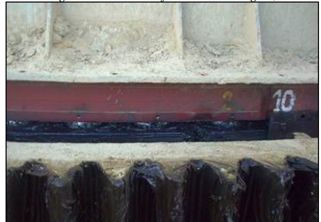
Figure 33. Visual control of relief of the rolling bodies of the radial-axial bearing;
