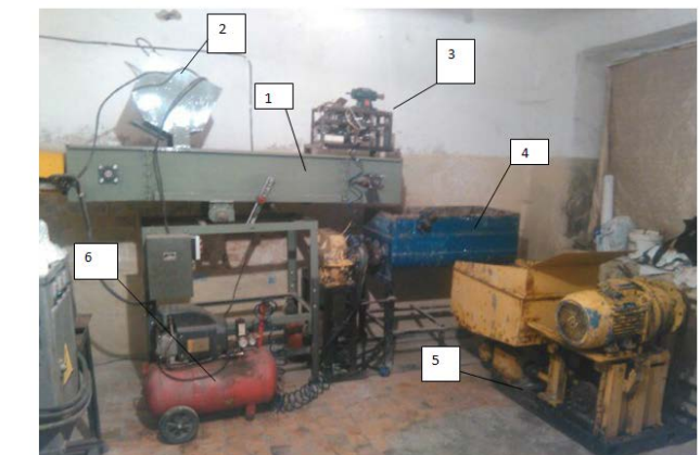
Fig.8. Technological set of small-scale equipment a) principal scheme of the technological set of equipment b) general view of the technological set of equipment 1 – Belt feeder; 2 – Belt feeder bunker; 3 – Synthetic fiber carver; 4 – Three-shaft concrete mixer; 5 – Concrete pump with disc valves; 6 – Compressor
