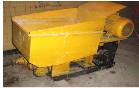
Fig. 4. Double-piston direct flow concrete pumps a) with conic valves; b) with disc valves.
