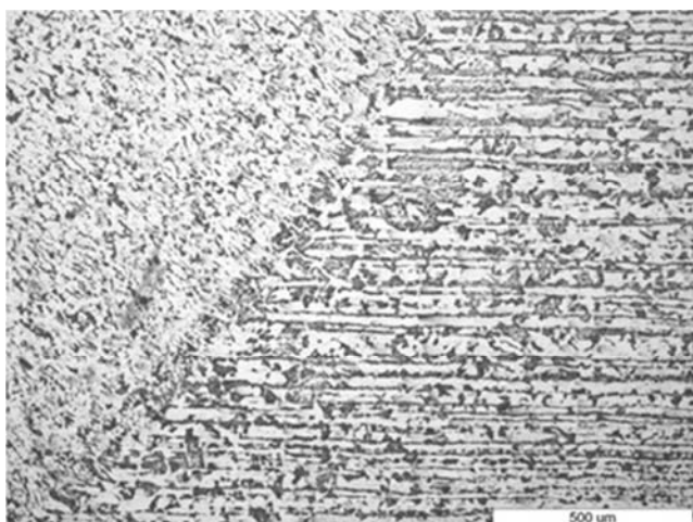
Figure 8 Fusion line and HAZ for welded sample S355J2+N, WN=0.88 , RF=0.2 , \sigma = \pm 0.009 , X200, nital.
