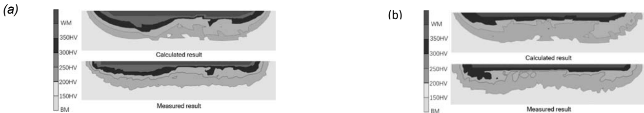
Fig. 10 Hardness distribution comparison of 1.5%Ni steel: (a) 1layer-3pass welding and (b) 6layer-21pass welding SI. 10 U poređenje raspodele tvrdoće za čelik 1.5%Ni: (a) 1 sloj-3 prolaza i (b) 6 slojeva-21 prolaz
