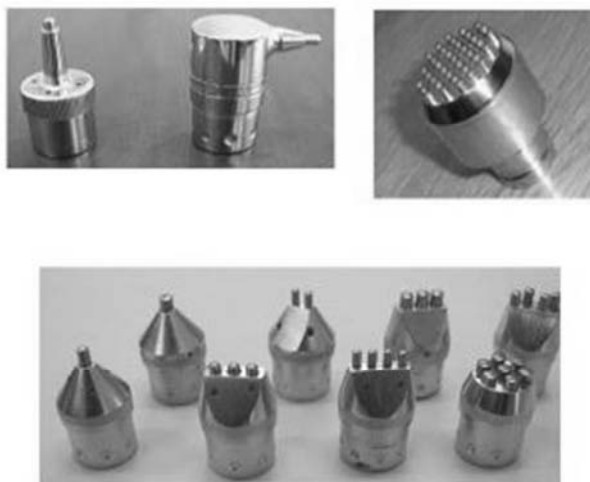
Figure 11. Examples of the replaceable interchangeable working heads developed for the ultrasonic peening of materials and structures.
