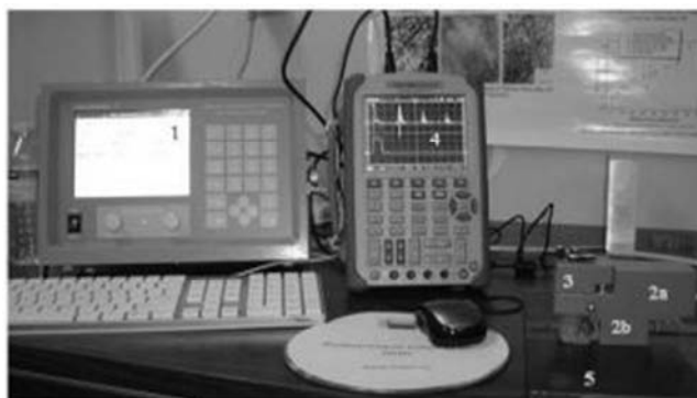
Figure 9. Ultrasonic Computerized Complex for residual and applied stress measurement. - Measurement unit UltraMARS with supporting software, (2a) – Preamplifier, (2b) – Magnetic holder, (3) – Transducer, (4) – Oscilloscope, (5) – Sample.
