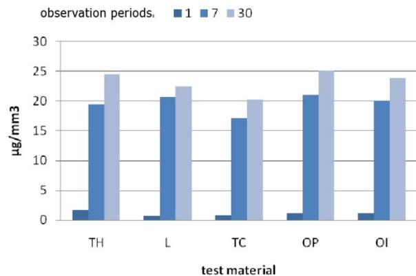
Figure 1. Mean values of water sorption after water storage
