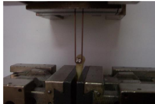
Figure 2. Dental sample placed in an electronic dynamometer
