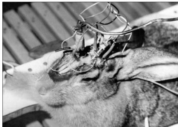
Figure 3. The figure shows simultaneous registration of EEG activity and activity of single neurons using microelectrodes implanted in deep subcortical brain structures on an experimental animal (rabbit) [8]
