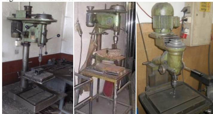
Slika 2. Bušilice koje nisu opremljene zaštitnikom oko prenosnog mehanizma (sopstveni izvor) Figure 2. Drilling machines not equipped with a safety gear around the transmission (Authors source)
