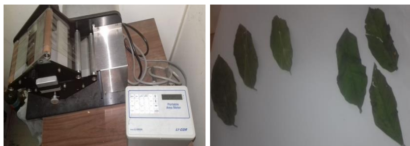
Fig. 4: Portable area meter model Li-COR Li30000A measured the area of lemon ( Citrus Limon ) and guavas ( Psidium guajava. L )
