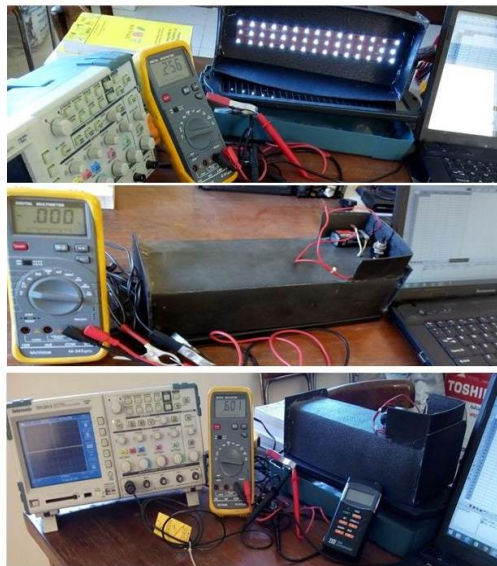
Fig.2. The developed solar leaf area meter and the instruments to measure the power and voltage
