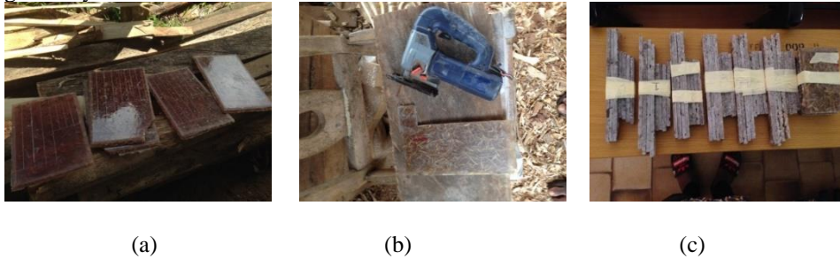
Plate 1. Picture of (a) cured composite, (b) Cutting of composite into test sample geometry and (c) Corn Stalk/Polyester Composite Test Samples ready for testing.
