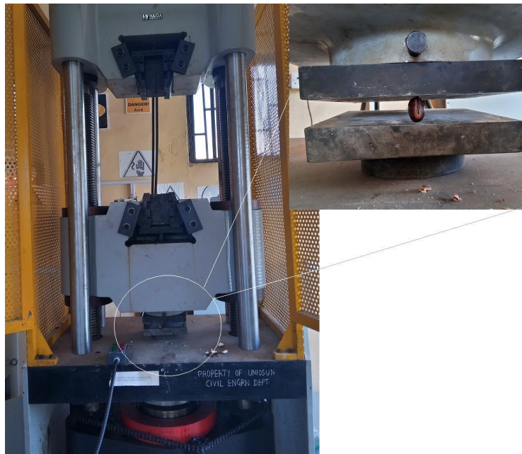
Figure 2. Placement of seed between the platens of Haida International- Mechanical Universal Testing Machine used in compression tests.
