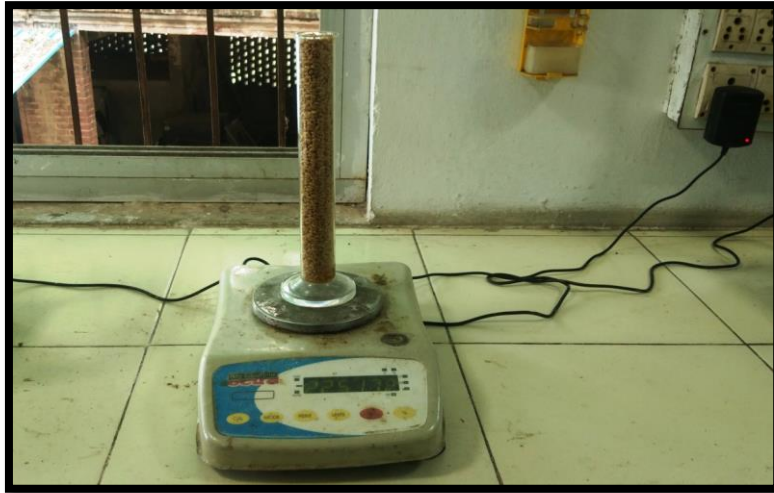
Fig. 3. Measurement of bulk density of wheat seed grain sample by measuring cylinder
