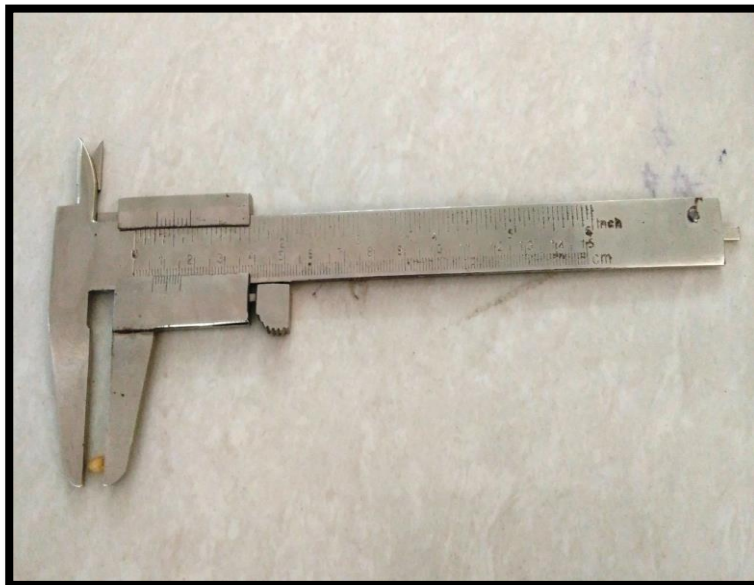
Fig. 4. Measurement of equivalent diameter and sphericity of wheat seed grain by calliper
