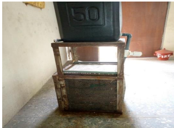
Fig. 1. Tomatoes stored in passive evaporative cooler (PEC)
