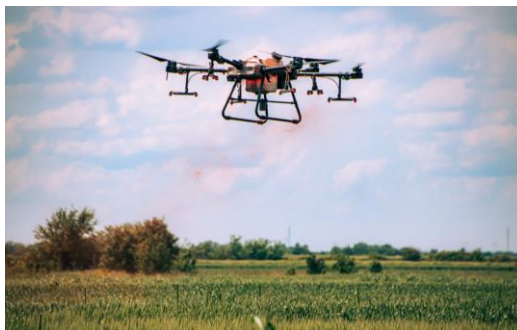
Figure 1. UAV system for pesticide application in wheat fields
