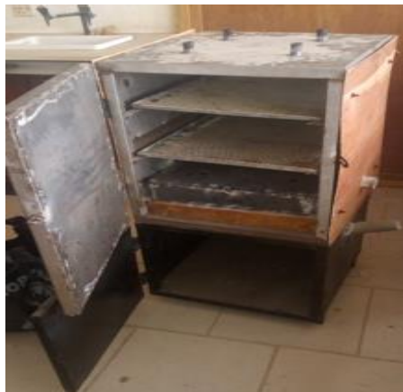
Plate 1. Fabricated indigenous multi-heat-source crop dryer
