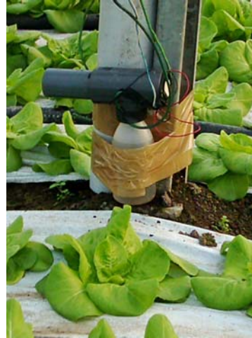
Sl. 4. Merenje temperature suvog i vlažnog termometra Fig. 4. Measurement with dry and wet thermometer
