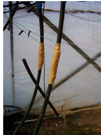
Sl. 5. Merenje temperature polazne i povratne vode za grejanje Fig. 5. Measurement temperature of inlet and outlet heating water
