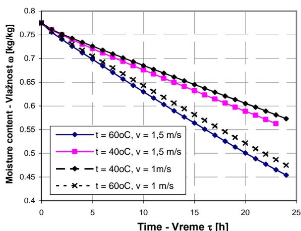
Fig. 5. Moisture content changing within convective drying
