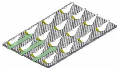
Fig. 2. Samples disposition on tray and air flow direction
