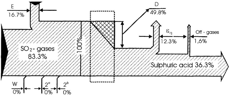
Fig. 5. Grassman's diagram of the process of making sulphuric acid by two-stage conversion: 2<sup>a</sup>, 2<sup>b</sup> - air; W-water; E-electric energy; D-internal exergy losses; ε<sub>q</sub>-heat exchange with environment.
