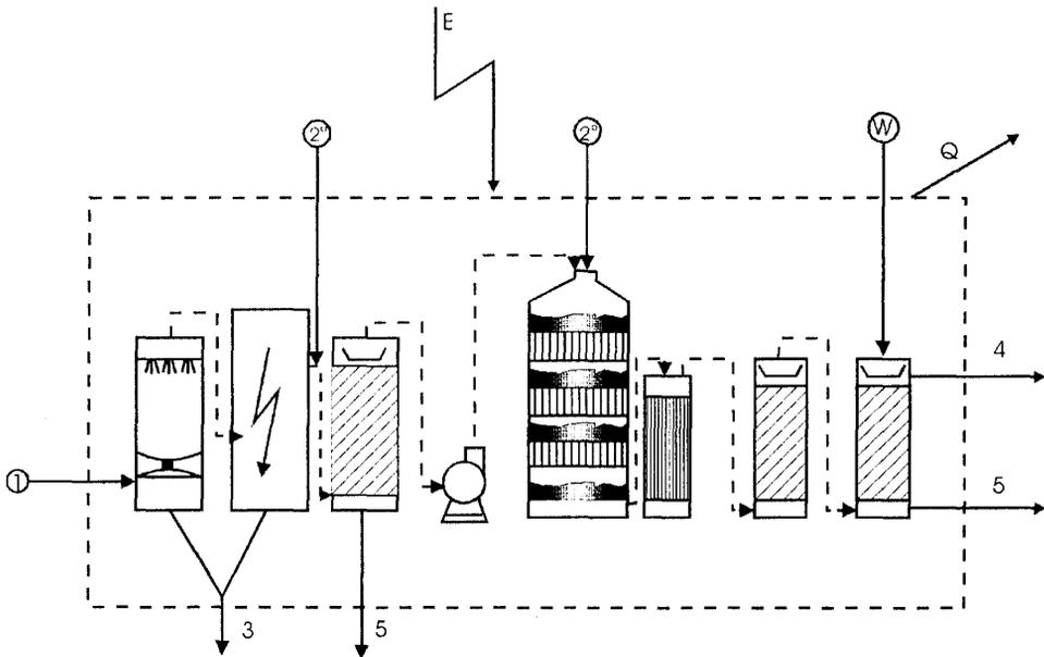
Fig.1. Chart of the process of making sulphuric acid by one-stage conversion:
