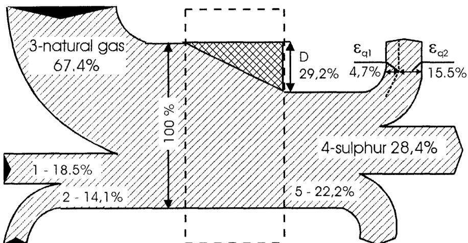
Fig. 6. Grassman's diagram of the process of making sulphur from SO<sub>2</sub>-containing gases: 1-SO<sub>2</sub>-containing gases; 2-energy from heating of SO<sub>2</sub>-gases; 5-off-gases; D-internal exergy losses;  $\epsilon_{q1}$ -heat exchange with environment;  $\epsilon_{q2}$ -heat discharged during the cooling of gases after the reduction column.
