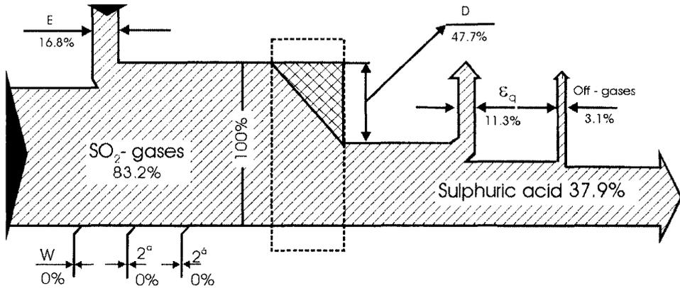
Fig. 4. Grassman's diagram of the process of making sulphuric acid by one-stage conversion: 2<sup>a</sup>, 2<sup>b</sup> - air; W-water; E-electric energy; D-internal exergy losses; ε<sub>q</sub>-heat exchange with environment.
