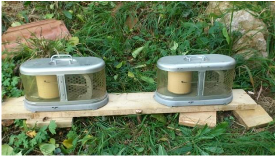
Figure 4 Thermograph and hydrograph positioned near the cracked wall
