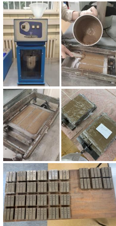
Figure 2 Preparation of mortar samples (2nd series - GSP)
