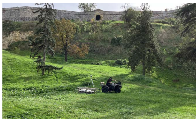
Fig. 10. Geophysical survey in the Lower Town, October 2023 – Malâ Mira HDR GPR motorized apparatus with RTK-GNSS receiver (source: GeoSphere Austria, Department of Near-Surface Geophysics)
