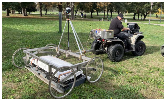
Fig. 10. Geophysical survey in the Lower Town, October 2023 – Malâ Mira HDR GPR motorized apparatus with RTK-GNSS receiver (source: GeoSphere Austria, Department of Near-Surface Geophysics)
