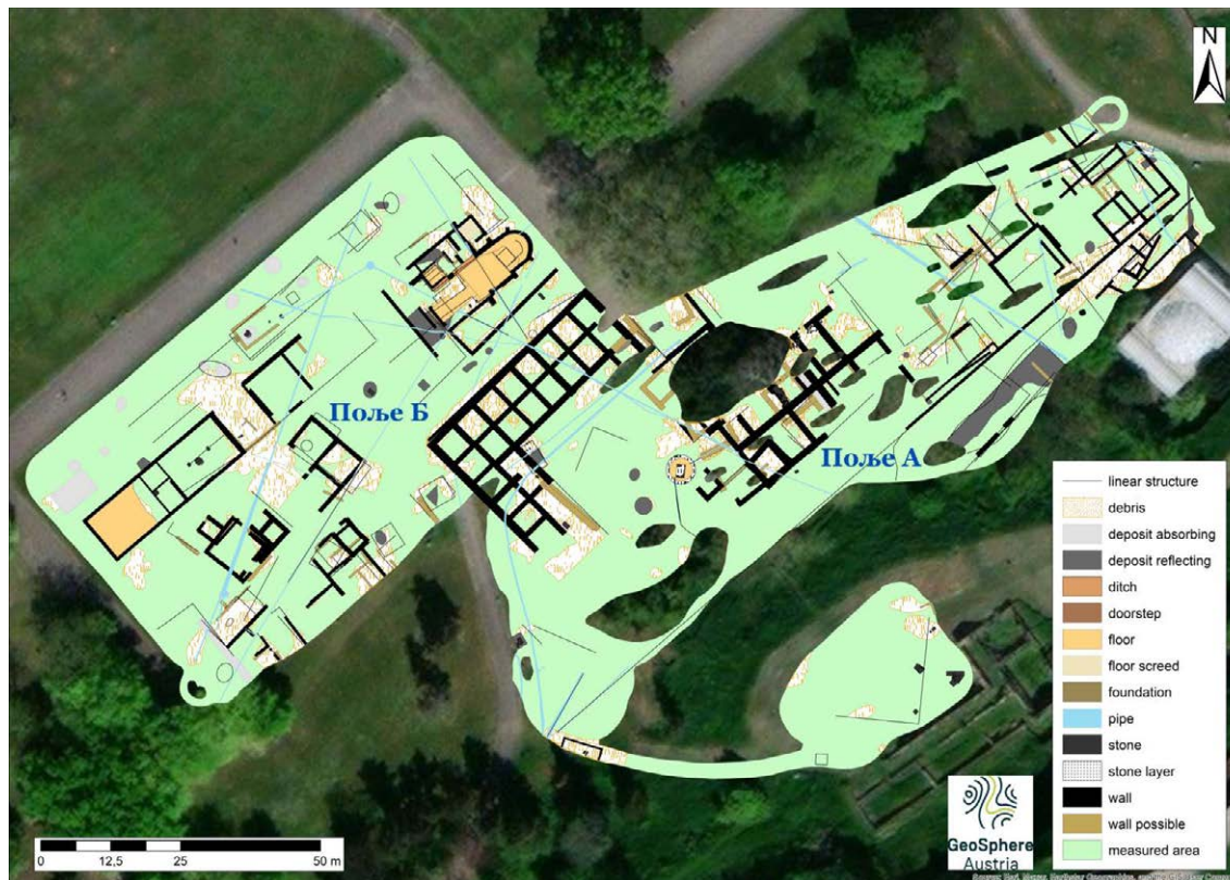
Fig. 12. Cumulative interpretation of all depth sections and magnetic prospection (source: GeoSphere Austria, Department of Near-Surface Geophysics)
