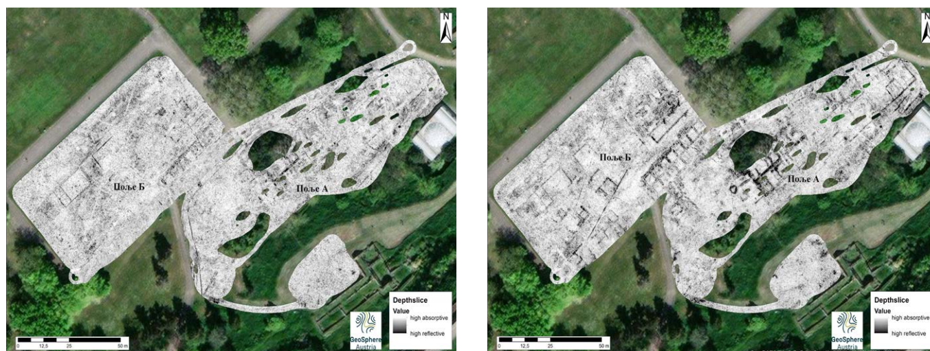
Fig. 11. Results of geophysical measurements at depths of 0.30–0.40 m (a) and 0.90–1.00 m (b) (source: GeoSphere Austria, Department of Near-Surface Geophysics)
