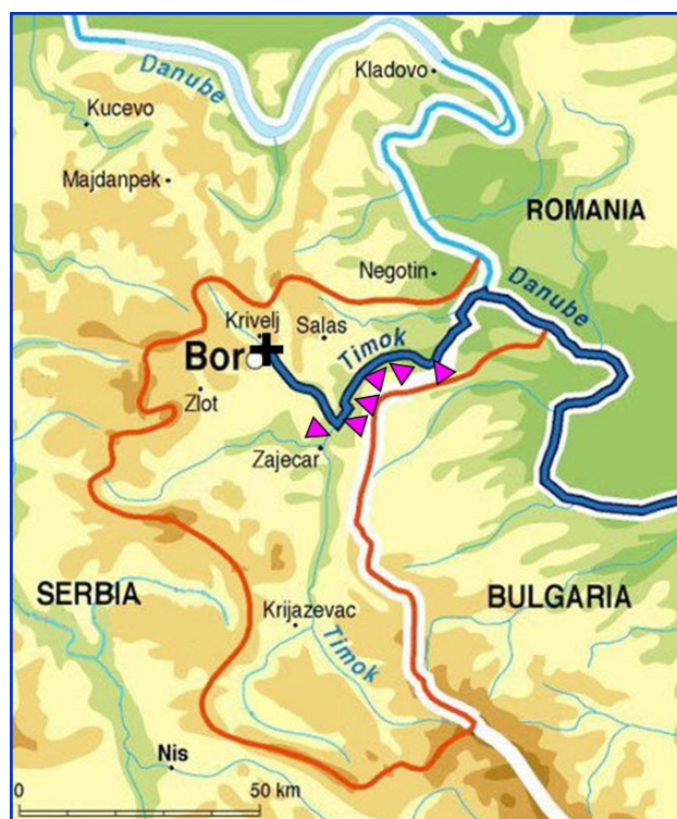
Figure 1. Study area. Red line denotes the Timok watershed, black cross marks the ore flotation facilities and the leaking tailing ponds. Polluted waterways are emphasized in dark blue, while purple triangles mark the major research sites.
