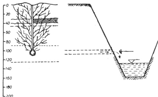
Fig. 8. - The scheme of mole's drainage
