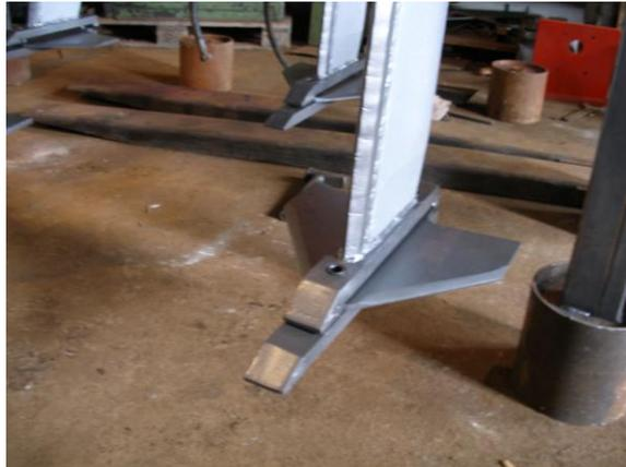
Fig. 9. - Working units of vibrating subsoiler VR-5(7)
