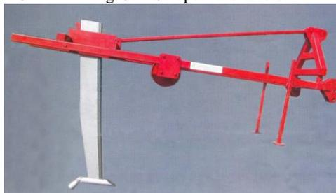
Fig. 7. - Vibrating subsoiler VR-5(7)
