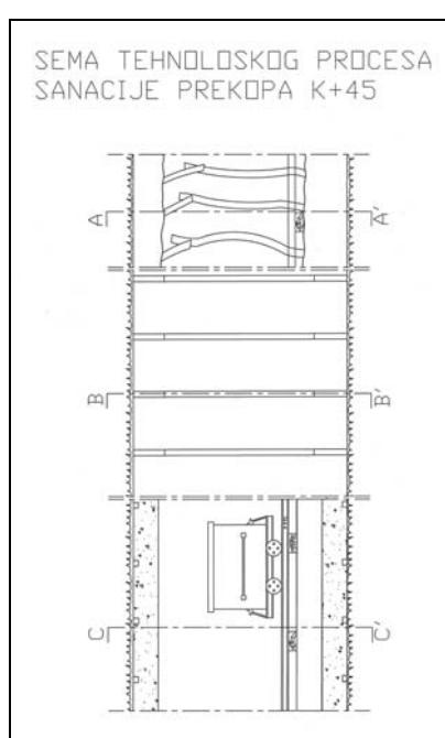
Reconstruction of the room is done through the following working operations: the extraction of deformed support, processing of profile to the designed size, loading of excavated material, and temporary supporting and dewatering.
