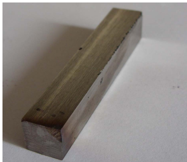
Figure 2. The image of the print on the sample for hardness testing by HRC method
