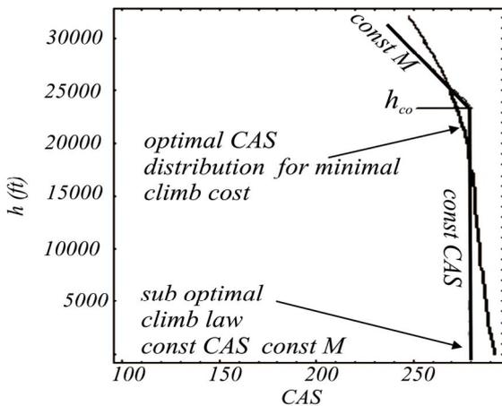
Figure 10. Adjustment of optimal CAS distribution with  $h$  with climb schedule: const CAS, const  $M$  and  $h_{co}$
