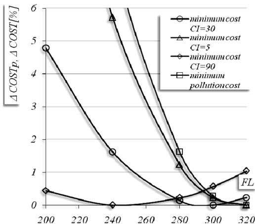
Figure 16. The percentage change of direct operating cost and pollution costs, in climb, with *FL*, for total *en route* flight
