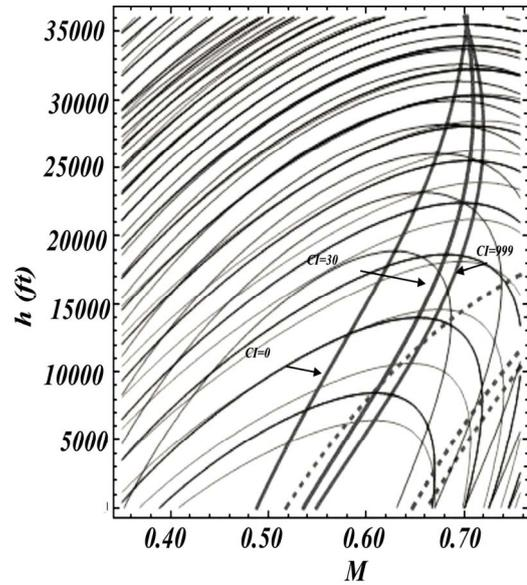
Figure 3. The contours of constant RCC and function of optimal  $M$  distribution for minimum RCC, with  $h$ , for minimum direct operating costs, for B737300 with CFM56 engines, for  $CI=0, CI=30$  and  $CI=999$
