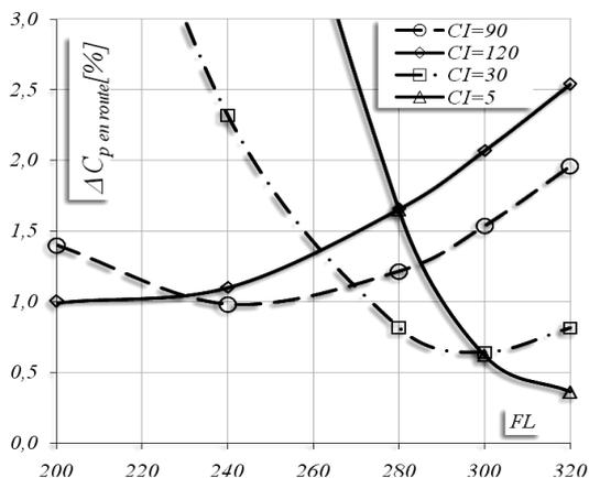
Figure 17. The percentage increase of direct operating cost for minimum pollution for *en route* flight
