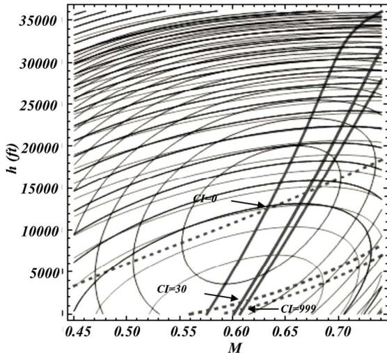
Figure 2. The contours of constant RCC and function of optimal  $M$  distribution for minimum RCC, with  $h$ , for minimum direct operating costs, for B767300 with PW4056 engines, for  $CI=0, CI=30$  and  $CI=999$
