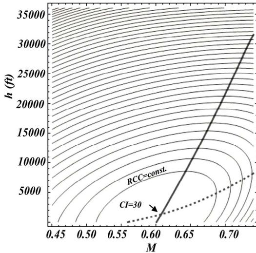
Figure 1. The contours of constant RCC and function of optimal  $M$  distribution for minimum RCC, for minimum direct operating costs, for B767300 with PW4056 engines, for  $CI=30$
