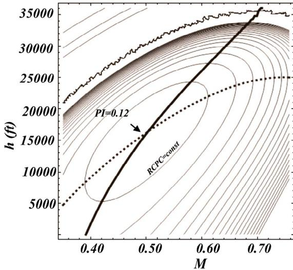
Figure 8. The contours of constant RCPC and function of optimal  $M$  distribution and optimal  $h$  distribution, for minimum RCPC, with  $h$  and  $M$ , for minimum pollution for B737300 with CFM56 engines in case of  $PI=0.121$
