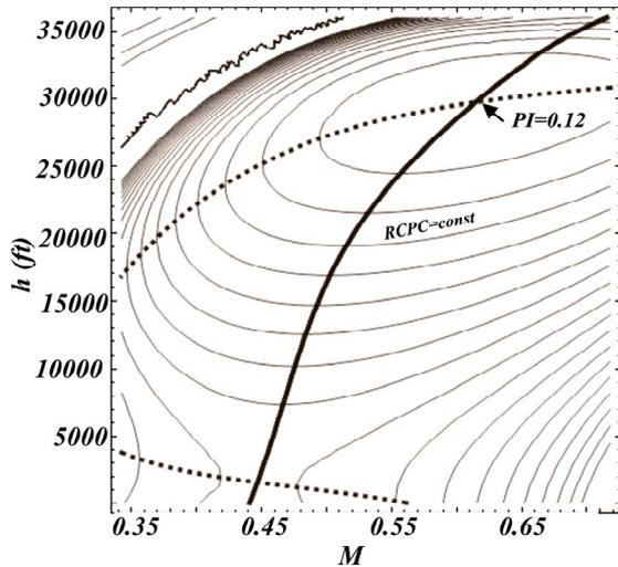
Figure 6. The contours of constant RCPC and function of optimal  $M$  distribution for minimum RCPC, with  $h$ , for minimum pollution for B767300 with PW4056 engines for  $PI=0.121$
