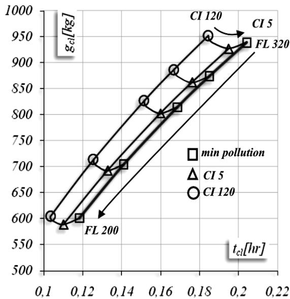
Figure 12. Mass of fuel and elapsed time in climb flight phase for different climb techniques
