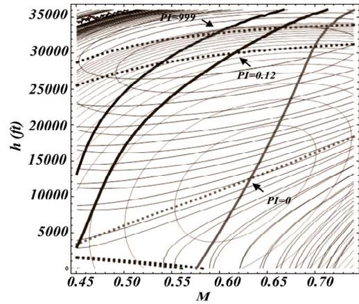
Figure 7. The contours of constant RCPC and function of optimal  $M$  distribution for minimum RCPC, with  $h$ , for minimum pollution for B767300 with PW4056 engines for  $PI=999$ ,  $PI=0.121$ ,  $PI=0$
