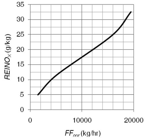
Figure 5. Relation between  $REINO_x$  and  $FF_{cor}$ , ICAO data bank for PW4056 turbofan engine
