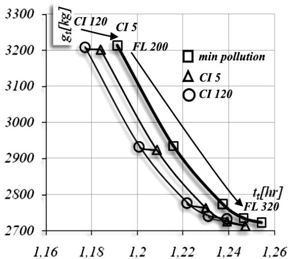
Figure 14. Mass of fuel and elapsed time for *en route* flight complete with different climb techniques
