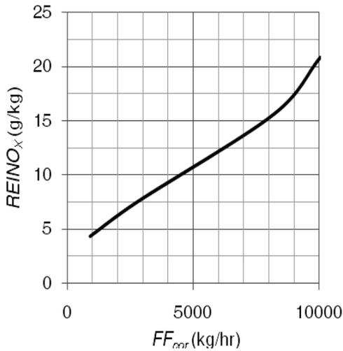
Figure 4. Relation between  $REINO_x$  and  $FF_{cor}$ , ICAO data bank for CFM 56 turbofan engine
