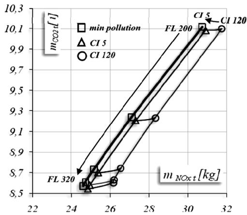
Figure 15. Mass of CO<sub>2</sub> and NO<sub>x</sub> emission in *en route* flight phase for different climb techniques
