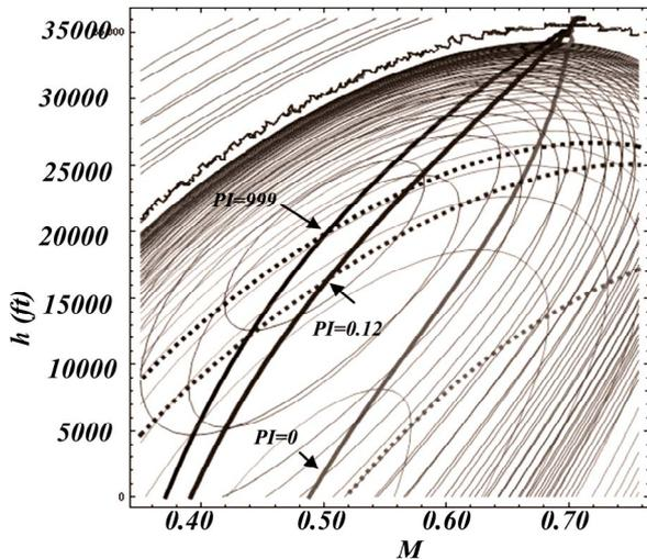
Figure 9. The contours of constant RCPC and function of optimal  $M$  distribution for minimum RCPC, with  $h$ , for minimum pollution for B737300 with CFM56 engines for  $PI=0.99$ ,  $PI=0.121$  and  $PI=0$
