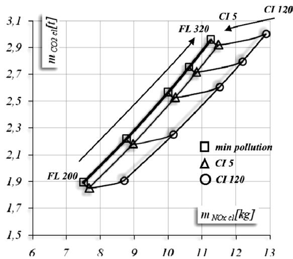
Figure 13. Mass of CO<sub>2</sub> and NO<sub>x</sub> emission for climb flight complete with different climb techniques
