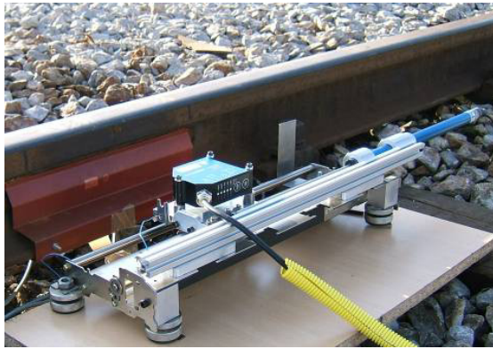
Figure 8. Laser system during positioning
