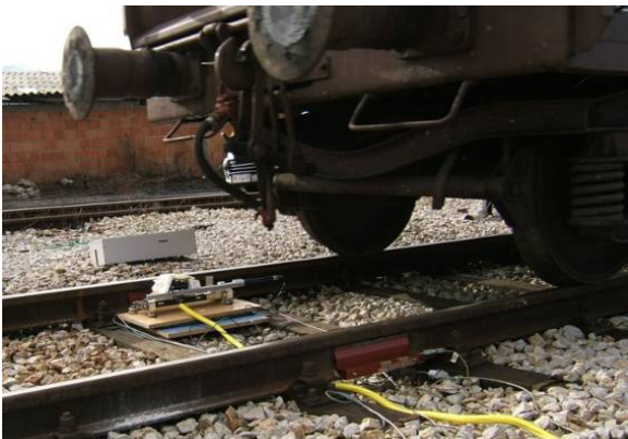
Figure 10. Trailing unit EMU 416-077 – angle of attack measurements [6]
