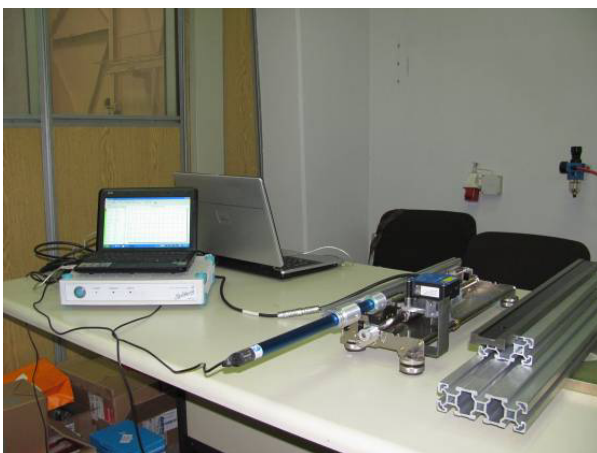
Figure 4. System for wheel to rail AOA measurements
