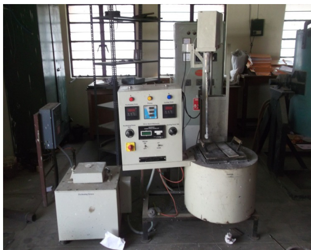
Figure 1. stir casting setup
