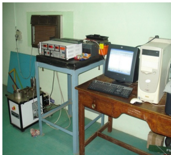
Figure 2. Pin on disc tribometer wear testing setup
