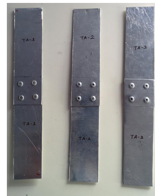
Figure 4. Riveted specimens for tensile testing
