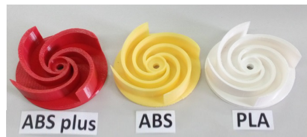
Figure 4. Impellers made from ABSplus, ABS, and PLA
