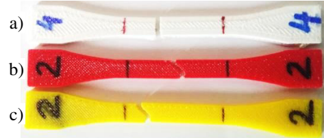
Figure 10. a) PLA, b) ABSplus and c) ABS specimens after failure
