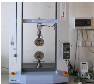
Figure 8. Testing machine for tensile and bending tests
