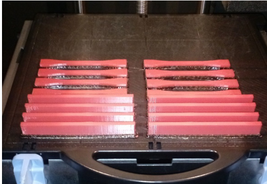
Figure 6. 3D printing of specimens in ABSplus using the Dimension Elite 3D printer platform.
