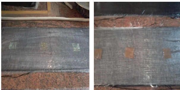
Figure 1. Introduction of Teflon plates in hybrid composite
