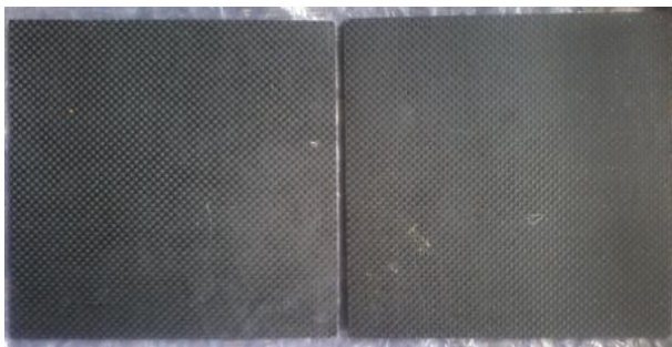
Figure 2. Finished glass-carbon/epoxy hybrid composite
