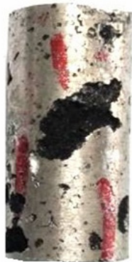
Figure 8. Show the AA2219 MWCNT powder cluster inside the machined cast samples.
