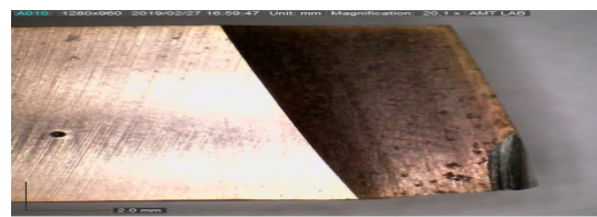
Figure 5. HSN2 tool after 1 st trial
