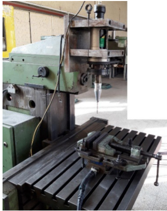
Figure 1. Experimental set-up of ultrasonic-assisted drilling process
