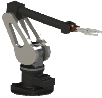
Figure 3. The adopted robotic system with 3 DOFs
