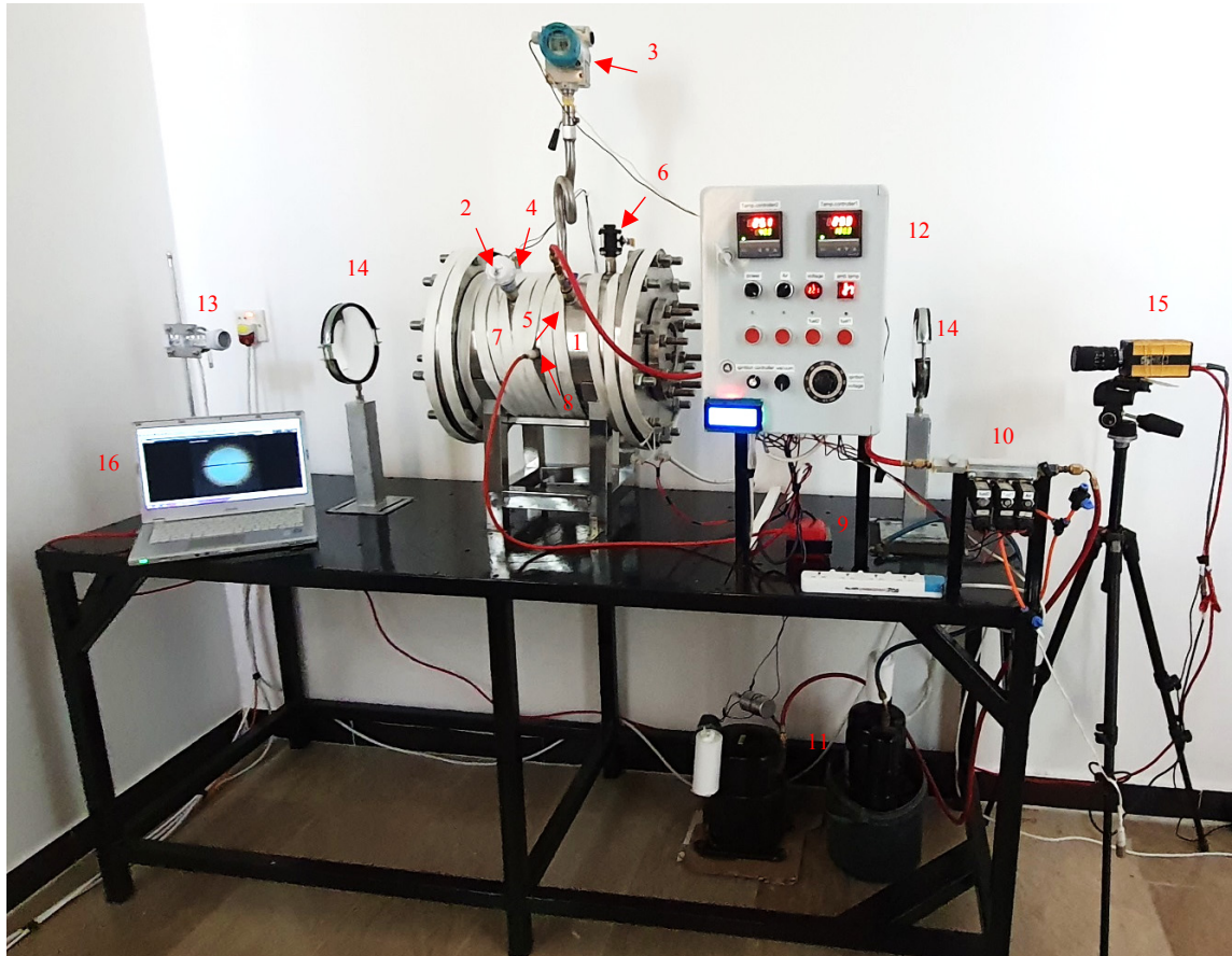
Figure 1. Photograph of the experimental apparatus used in the study. (1) Combustion chamber, (2) Thermocouple, (3) Pressure transmitter, (4) Liquid fuel injection valve, (5) Inlet valve, (6) Exhaust valve, (7) Electrical heating tape, (8) Sparking ignition electrodes, (9) Ignition burner transformer, (10) Injection unit, (11) Vacuum pump, (12) Electrical control board unit, (13) Light Source, (14) Two lenses (15) High-speed camera, and (16) PC computer.
