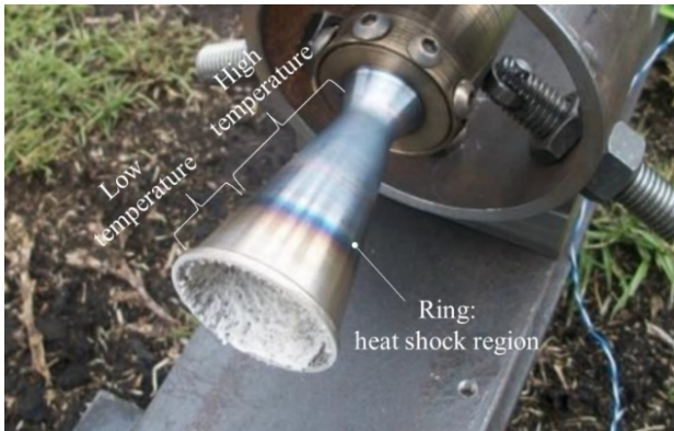
Figure 1. The conical nozzle was subjected to experimental static testing by Riveros and Rodriguez [16].
