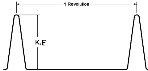
Fig. 1a: Pulsating bending load
