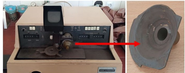
Figure 2. Micro Automation device for cutting silicon wafers (left) with a fractured protective cover (right)
