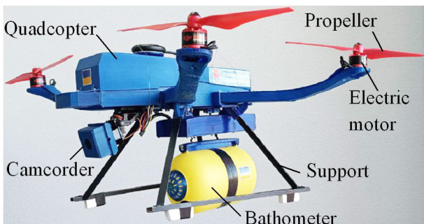
Figure 1. Prototype drone for water sampling
