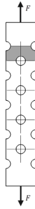
Figure 7. A separated strip from the sample with a triangular arrangement of openings
